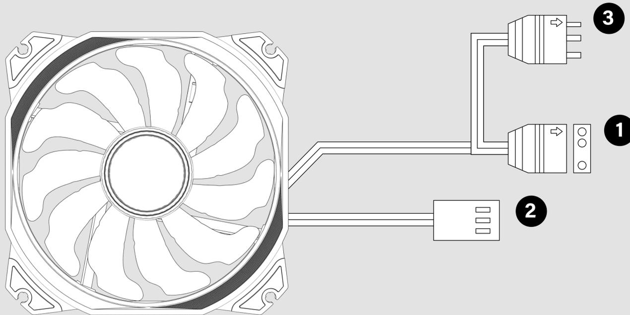
**1** 5v ARGB connector to motherboard/fanhub controller
